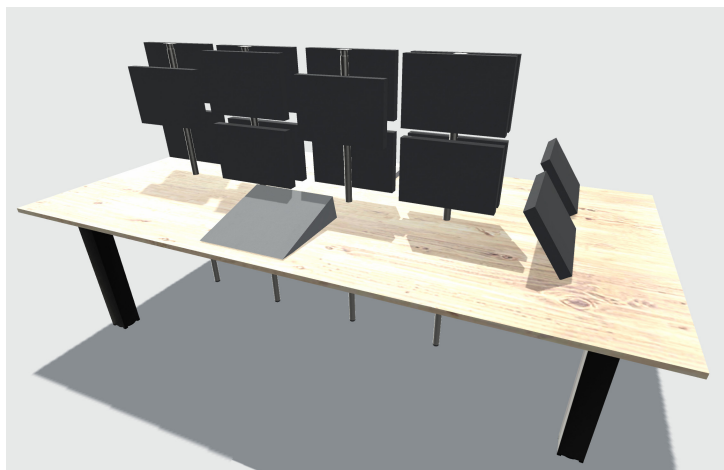
Figure 3.4: View of the proposed workplaces within the Control Room - From left to right: Score Assistant, Director, opt. Vision Engineer, Production Engineer (not proportional - no scale - draught idea only).
